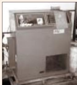
On-site, batch antifreeze recycling units are available with filtration or distillation recycling technology.
